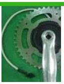
Chain Wheel Torque Sensor startup immediately according to the size of pedaling force and output linear propotionally Disadvantages:
